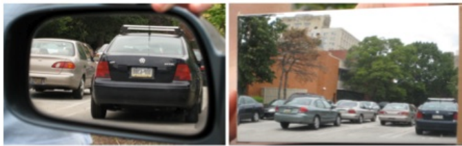
Figure 4. On the left we see a parking lot via a conventional flat driver-side mirror. On the right is a view of the parking lot with the mirror designed by the author.
